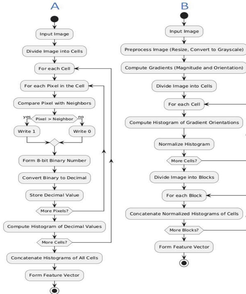
FIGURE 1. - Implementation step diagrams: A: LBP, B: HOG
